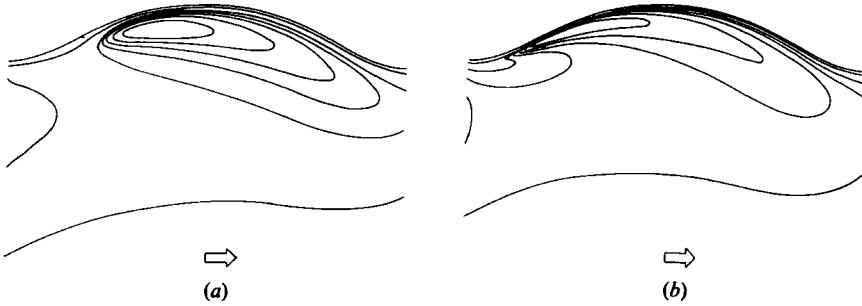
FIGURE 18. Contour plots of turbulent kinetic energy: (a) Re_H = 30000 ; (b) Re_H = 115000 .
